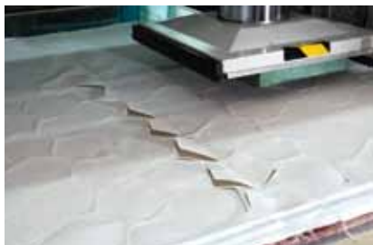
After the fabric was stretched and laminated, panels are machine-cut to ensure they are all the same size.
