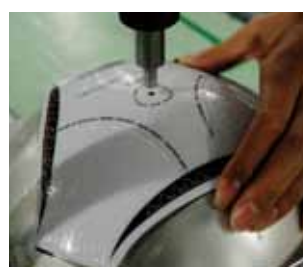
The valve hole is punched and four panels each are used to form the two ball halves. The two halves are again weighed and the valve centred.
