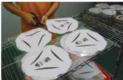
Logos are heat-transferred to the TPU sheet, which is cut in 8 pieces, on a print conveyor. They are then inspected. The 11 colours are printed with an underglass process
