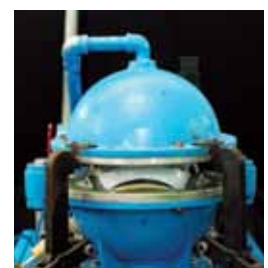
The carcass and ball halves are thermal-bonded in air-pressure and heated moulds. Balls are chilled and stored 24hrs.
