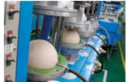
After the bladders are inserted and the valves affixed with glue, the carcasses are inflated and shaped to check roundness and seams.
