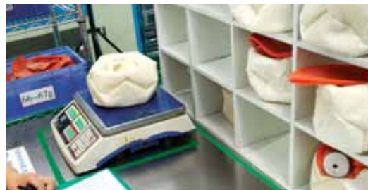
Once the panels are stitched, the carcasses are weighed to ensure that all weigh the same. Bladders are weighed separately and with the carcasses to ensure uniformity.
