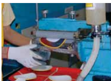
3D EVA panels, UV-treated to cleanse them, are vacuum bonded at high-frequency with the TPU, and trimmed. The backs of the panels are automatically glued.
